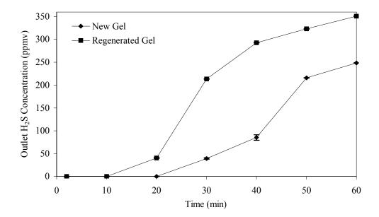
Figure 5.4: Outlet H<sub>2</sub>S concentration over time from both new and regenerated 1000 g silica gel tests, GC analysis with SRI 8610, 10 ppmv H<sub>2</sub>S detection limit
