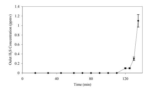
Figure C.2: CVHS Test #2, outlet H<sub>2</sub>S concentration, 10 L/min 1000 ppmv H<sub>2</sub>S dry landfill gas, 1000g of SulfaTreat®, results obtained with hand pump
