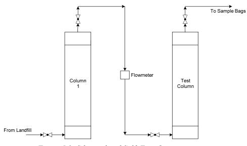
Figure 5.2: Silica gel and SulfaTreat® testing system
