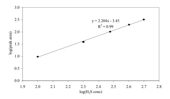
Figure 4.6: Least-Squares Linear Fit for FPD calibration, SRI 8610, 15 m column, 100-500 ppmv H<sub>2</sub>S
