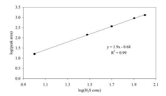
Figure 4.5: Least-Squares Linear Fit for FPD calibration, SRI 8610, 15 m column, 10-100 ppmv H<sub>2</sub>S
