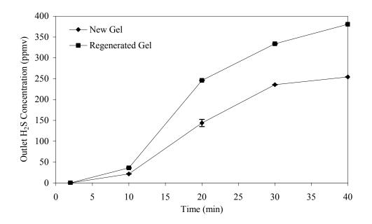
Figure 5.3: Outlet H<sub>2</sub>S concentration over time from both new and regenerated 500 g silica gel tests, GC analysis with SRI 8610 FPD, 10 ppmv H<sub>2</sub>S detection limit
