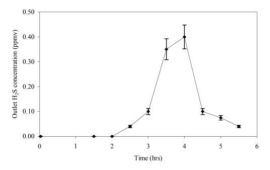
Figure 5.5: Outlet  $H_2S$  concentration, 5 L/min 500 ppmv  $H_2S$  landfill gas, 1000g of SulfaTreat<sup>®</sup>, results obtained with hand pump, 0.2-3 ppmv  $H_2S$  tubes,
