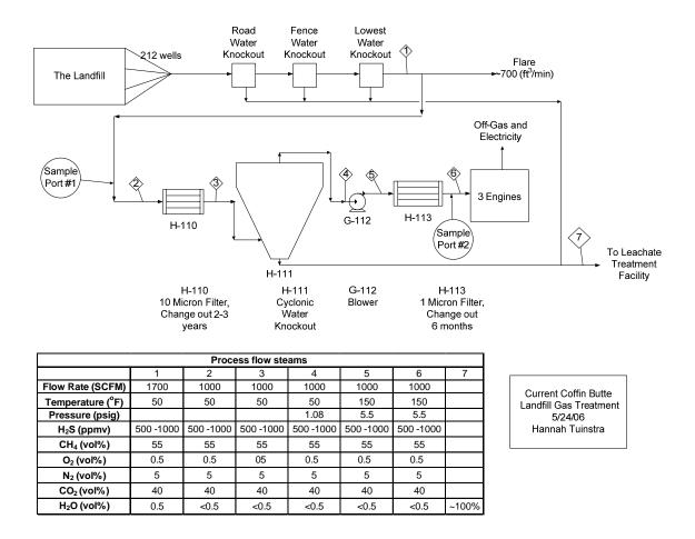
Figure 2.1: Process Flow Diagram for the Gas Recovery Plant at Coffin Butte Landfill
