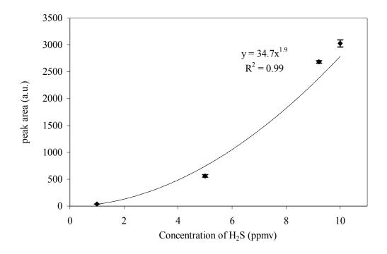
*Figure 4.7: Non-linear FPD calibration, SRI 8610, 60 m column, 1-10 ppmv H*<sub>2</sub>*S*
