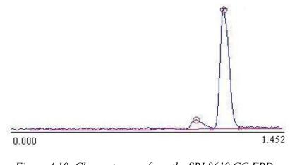
Figure 4.10: Chromatogram from the SRI 8610 GC FPD, to determine H<sub>2</sub>S concentration,
