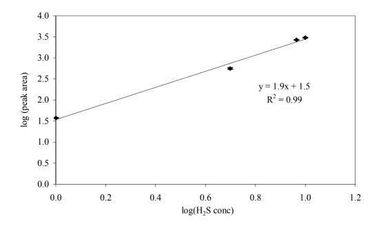
Figure 4.8: Least-Squares Linear Fit FPD calibration, SRI 8610, 60 m column, 1-10 ppmv H<sub>2</sub>S
