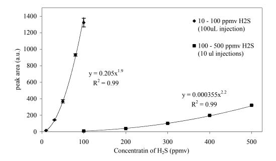
Figure 4.4: Non-linear FPD calibration, SRI 8610, 15 m column, two different injection sizes for different concentration ranges
