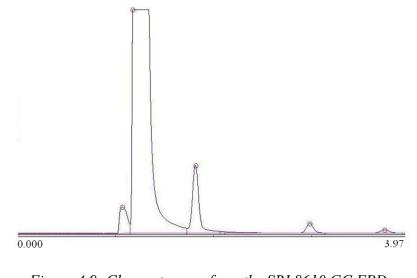
Figure 4.9: Chromatogram from the SRI 8610 GC FPD, to determine non-H<sub>2</sub>S sulfur compound concentration, 60 m column, 1 ppmv H<sub>2</sub>S detection limit, 1 mL injection of untreated landfill gas June 2006
